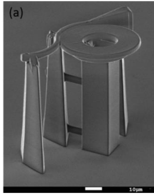
Free-standing microring resonator and the coupling waveguide Osellame et al., Lab Chip 19, 1985-1990 (2019)
