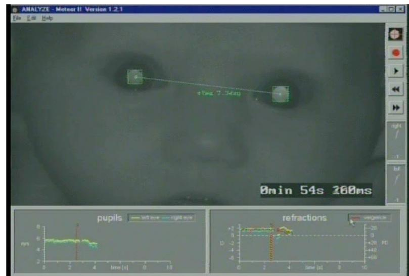
Eccentric photorefraction and Purkinje image eye tracking, at 25Hz or 50Hz. (PowerRefractor 1 or 3)
