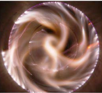
Rotating Non-Equilibrium Gliding Arc Plasma Disc for Enhancement in Ignition and Combustion
