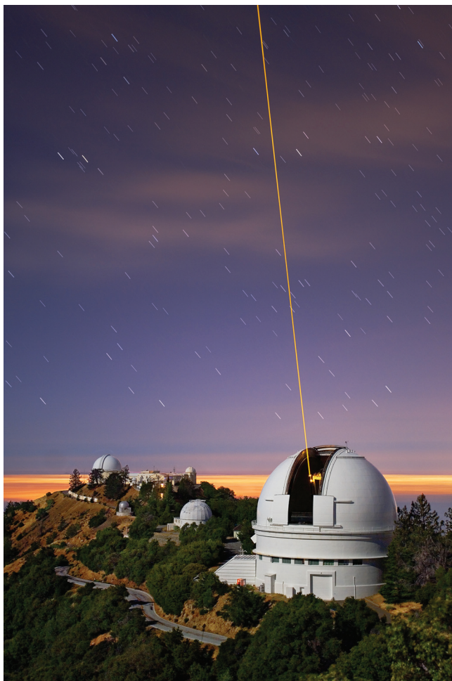
▲ Fig. 5. A laser guide star tuned to the wavelength of sodium atoms in the atmosphere, providing information on atmospheric turbulence to allow for adaptive optics to compensate and enable improved telescope resolution. (©Laurie Hatch.)
