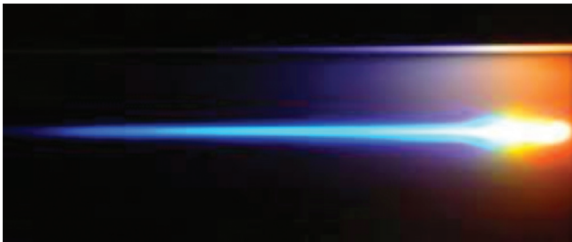
▲ Fig. 4. Supercontinuum generation using a prism to disperse the colors in the pulse. (Image courtesy of [7]. © 2008 SPIE, image credit: E. Goulielmakis, reprint_permission@spie.org.)
