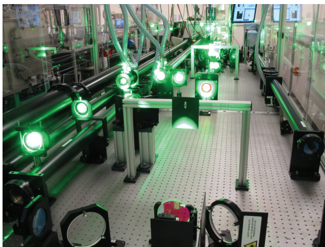
▲ Fig. 3. One of the two Gemini amplifiers at Rutherford Appleton Laboratory, showing, in the center, a green-laser-pumped Ti:sapphire crystal 90 mm in diameter and 25 mm thick. With 60 J of pump energy the system has generated 25 J of output energy in a 30 fs pulse. (STFC Gemini Laser Facility/Chris Hooker).
