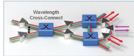
◀ **Fig. 3.** Evolution of reconfigurable, wavelength routed optical networks employing reconfigurable optical add/drops (ROADMs) and optical cross-connects.
