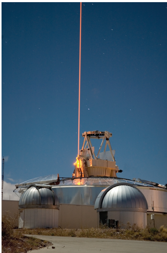
▲ Fig. 4 The Air Force Starfire Optical Range for lidar and laser guide star experiments is tuned to the sodium D2a line and used to excite sodium atoms in the upper atmosphere. This provides what is essentially a point source of light in the mesosphere to use for adaptive optics to remove blurring of ground based imaging due to atmospheric turbulence.
