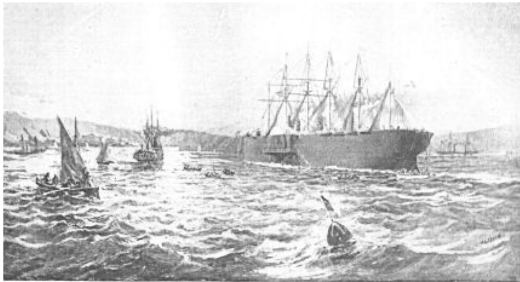
THE "GREAT EASTERN" COMPLETING THE LAYING OF THE SECOND ATLANTIC CABLE IN TRINITY BAY, NEWFOUNDLAND, JULY 1866. (By permission of Sir Charles Bright, F.R.S.E.)
