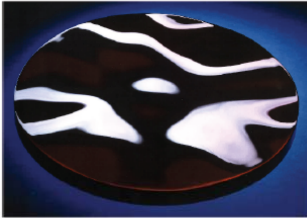
Typical TV lens profile – aspheric departure about 4mm
