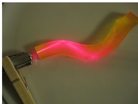
Figure 4 – Gelatin “optical fiber”. Note the total internal reflection where the laser beam strikes the gelatin-air boundary.
