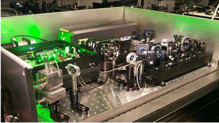
Original 800 MHz Ti:sapphire ring laser based frequency comb
