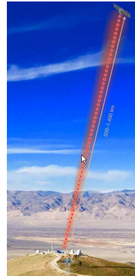
Satellite-mediated QKD, WCS 1-10 kbps, QBER 1%; trusted satellite. Liao et al. PRL (2018)
