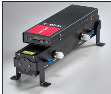
1ppm, 35cm + external pump, 1.9kg, 2W
