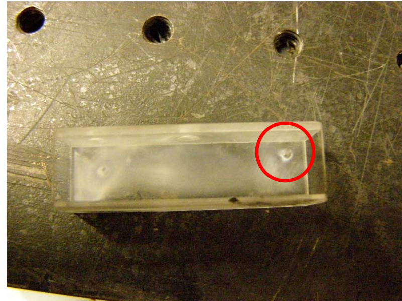
Damaged spot on the cuvette surface. Laser intensity was 1 MW/cm 2 .
