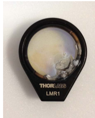
Tantala-silica damage at 2.5 \text{ MWcm}^{-2}
