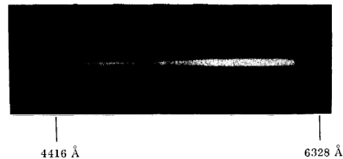
FIG. 2. (a) Continuum generated in the fiber waveguide with a broad-band Coumarin 120 dye laser as the pump.
