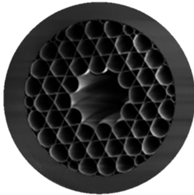
Scanning electronic microscope (SEM) image of the fiber
