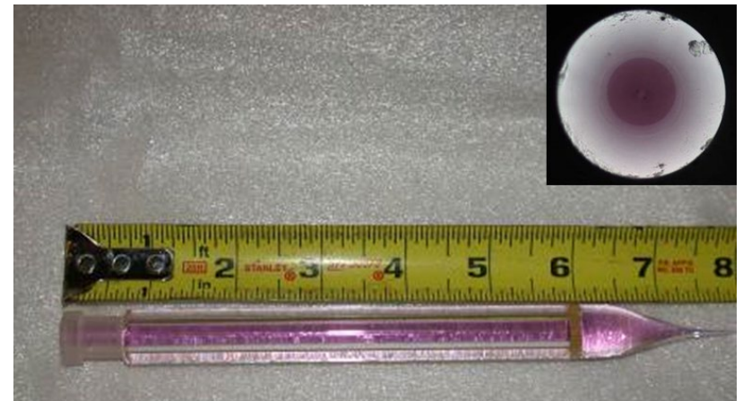
Nd:phosphate core sleeved inside passive phosphate glass cladding tube
