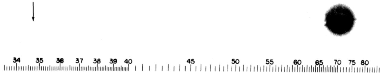
FIG. 1. A direct reproduction of the first plate in which there was an indication of second harmonic. The wavelength scale is in units of 100 Å. The arrow at 3472 Å indicates the small but dense image produced by the second harmonic. The image of the primary beam at 6943 Å is very large due to halation.
