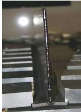
Straight near net shape Ti thin wall
