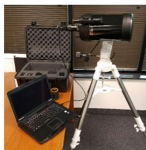
DELTA system with example outputs of differential jitter measurements and calculated C_n^2 profiles THE AIR FORCE RESEARCH LABORATORY
