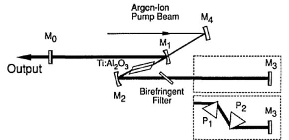
Fig. 1. Schematic of the cavity configuration for self-mode-locked Ti:Al<sub>2</sub>O<sub>3</sub> laser. The inset shows the intracavity prism sequence for dispersion compensation.
