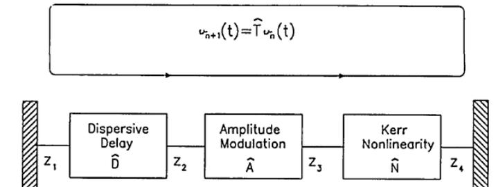
Fig. 1. Schematic of the solitary laser.
