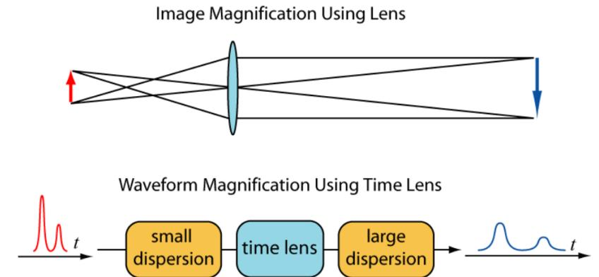
Picosecond structures are stretched to the nanosecond scale and measured using a fast oscilloscope
